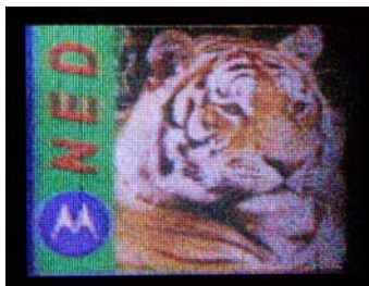
Figure 1: A 4.6-inch display using the emission properties of millions of CNTs from Motorola’s Nanoemissive display (NED) group.
